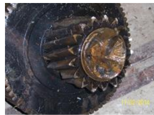
Fig4. Shaft is broken by fatigue failure. Fig5. Bearing was pushed progressively out the casing.
