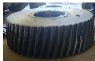
Fig6. Spur gear teeth damage. Fig7. Broken teeth damage.
