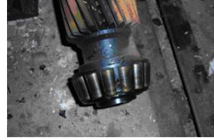
Fig2. Pinion surface polishing. Fig3. Bearing surface failure.
