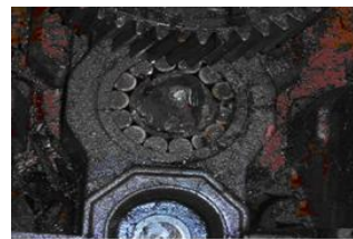
Fig4. Shaft is broken by fatigue failure. Fig5. Bearing was pushed progressively out the casing.
