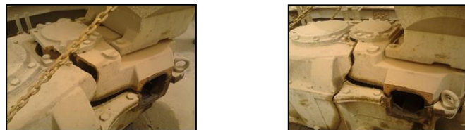
Fig1. Gear box top cover casing is broken into two parts.
