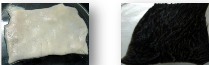
Fig4. Enzymatic dehairing by B. subtilis protease on left, control is on the right (without protease)
