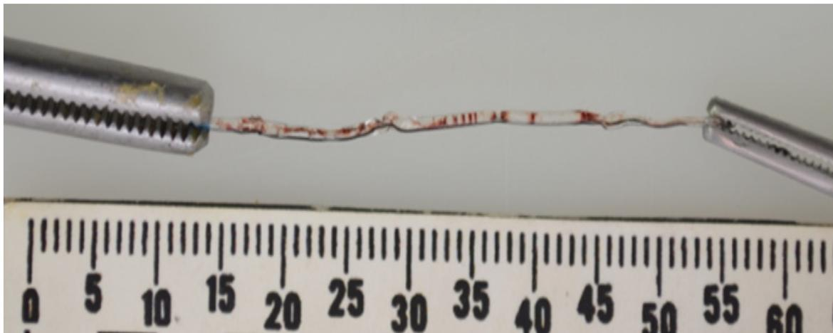
**Fig. 2.** *Unfolded epidural catheter fragment*
