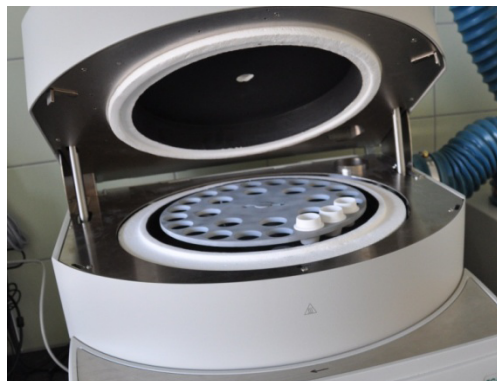
Fig3. TGA instrument with open cover an gravimetric measurements
