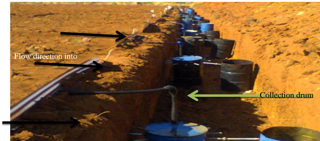
Plate 1: Runoff collection system
