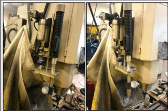
Fig. 5 Original GMAW Arm Mount Configuration
