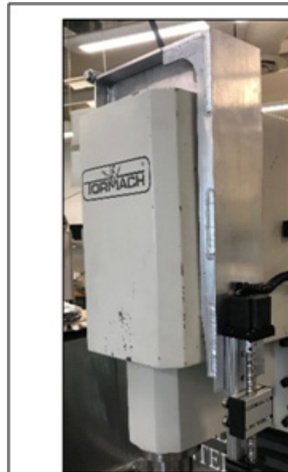
Fig. 7 New Mounted Aluminum GMAW Arm Mount
