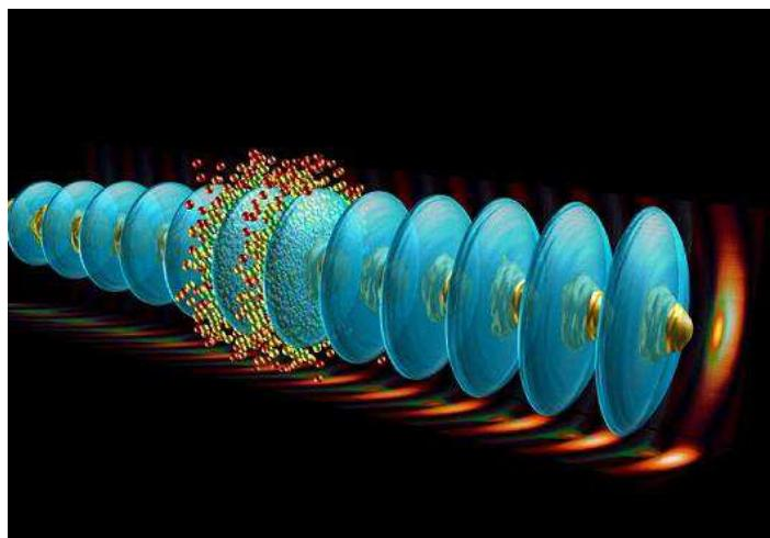
Fig. 8. Illustrates Surfing in the particle accelerator: In the AWAKE experiment, the protons (bullet-like structures) drive a plasma wave (elliptical structures) that accelerates electrons to high energies (small spheres). [13]
